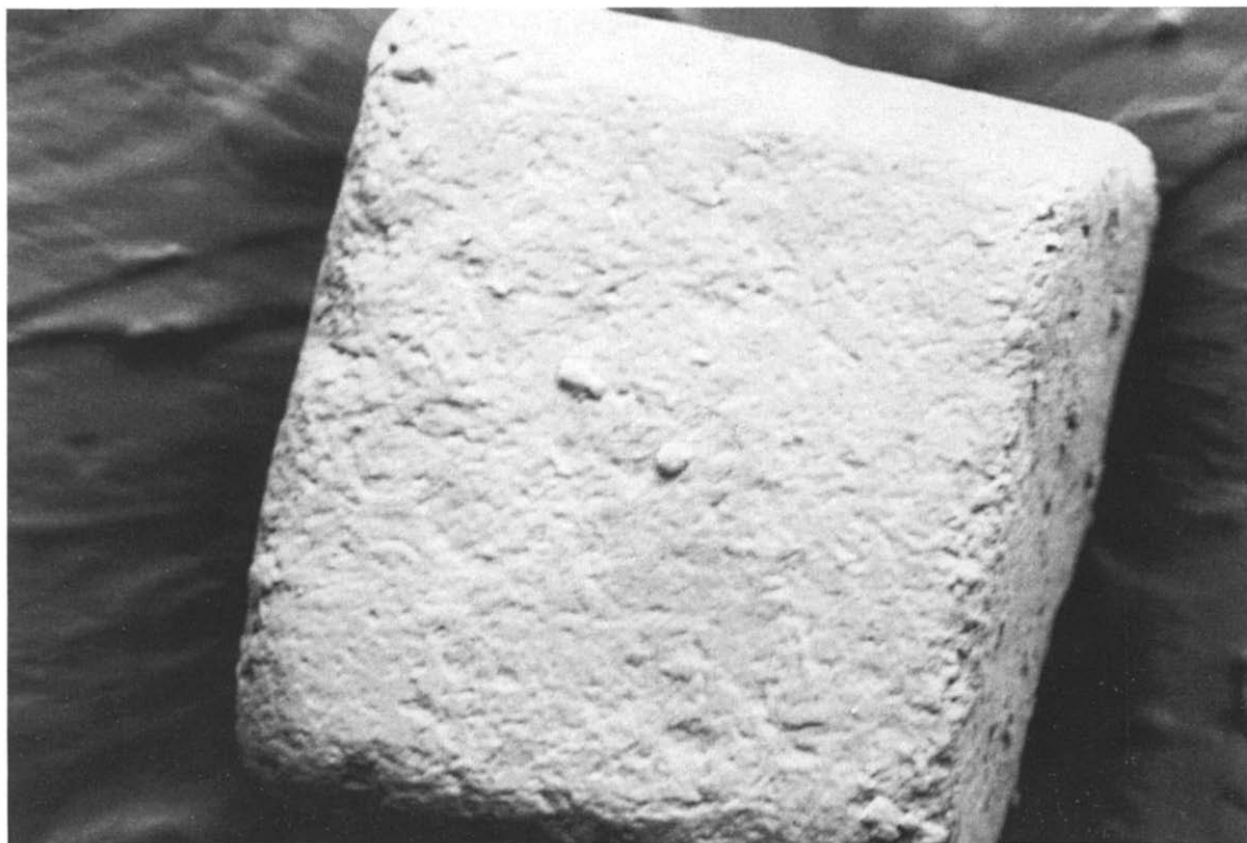
Fig. 4. SEM photomicrograph of a typical particle of sodium chloride \times 200 .
